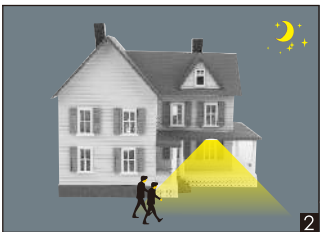
With insufficient ambient light, then sensor switches on the lamp when motion is detected.
